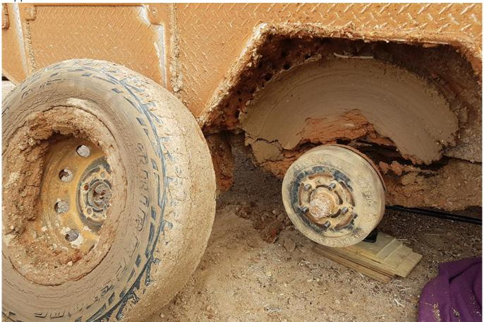
It's unlikely for two sets of bearings to collapse, so Kev only keeps one set of wheel bearings for one wheel in his kit. Credit: Kevin Leslie
