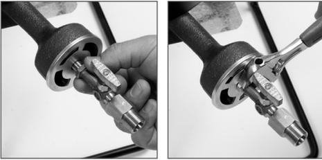
2. Align the male end fitting on the Gas Control Assembly to the venturi tube on the burner and screw in the internal thread on the burner. Use an adjustable spanner to tighten until tight.
