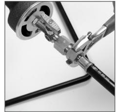
3. Attach the other end of the hose with the regulator to the gas cylinder, tightening using the two finger support posts.
