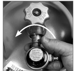
4. Check that gas control on cooker is turned "OFF", then turn the cylinder gas valve on in an anti-clockwise direction for one full turn and then check the connections for leaks with soapy water.
