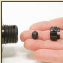
Insert new seal in orientation shown
