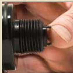
Re-install retainer and seal
