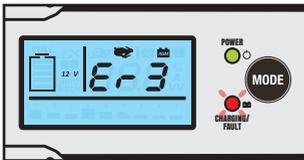
**Er3 - Red LED Slow Blink**: Fault code during initial charge step. Battery voltage doesn't reach a normal condition for charging.
