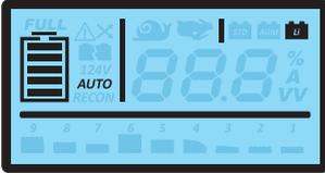
Our Lithium Battery Activation Mode lets our charger know that the battery being charged is in this Under Voltage Protection Mode.
