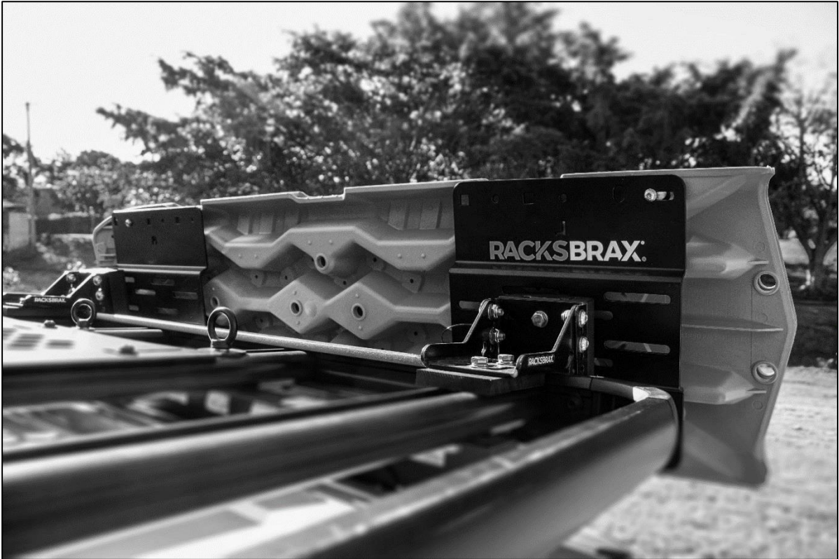
Figure 3 HD Accessory Plate Gen 2 mounted to transverse bars on a roof rack platform.
