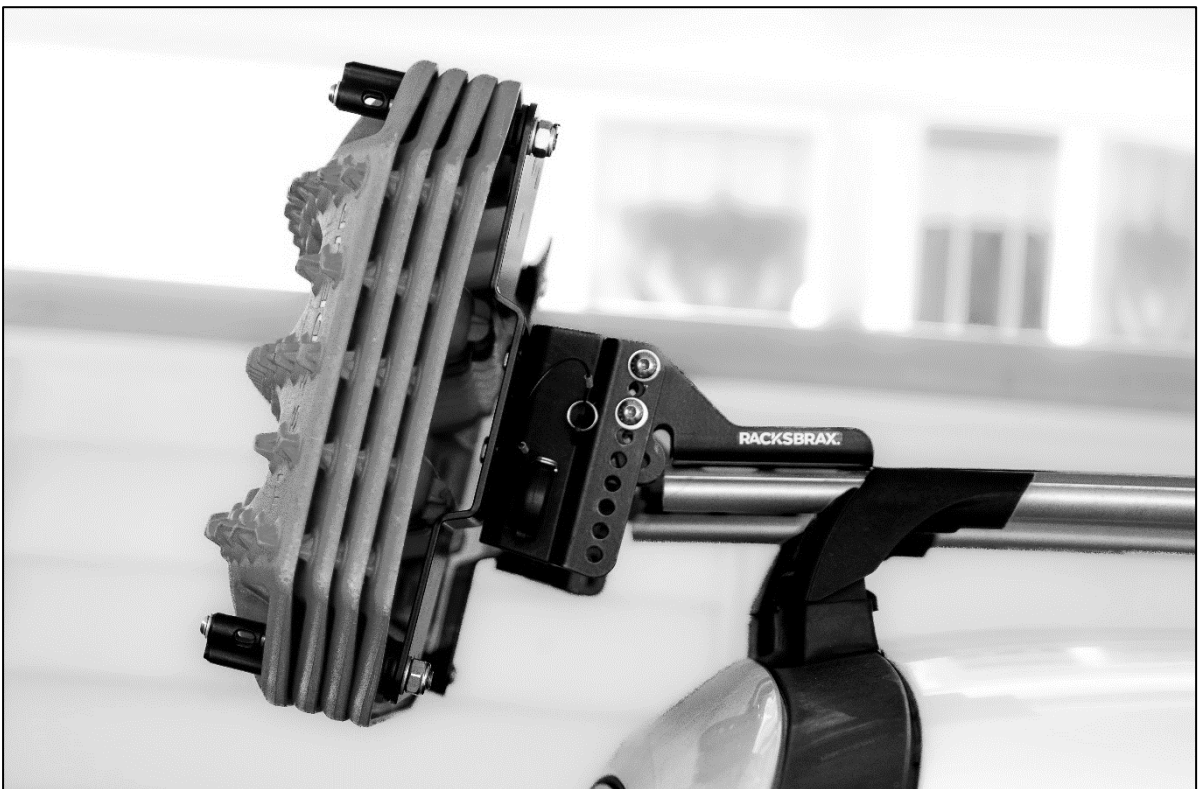
Figure 4 HD Accessory Plate Gen 2 mounted on roof aero style rack bars.
