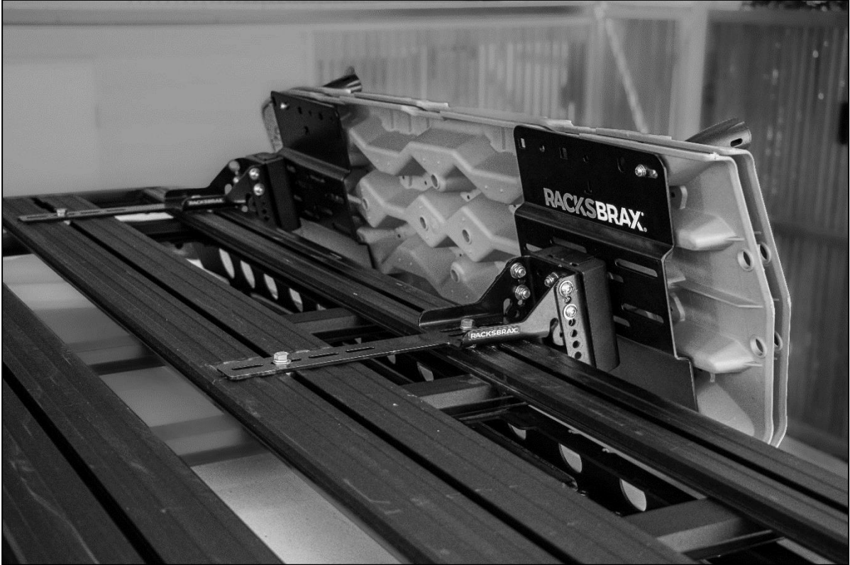
Figure 5 HD Accessory Plate Gen 2 Mounted to a platform rack with longitudinal slats.
